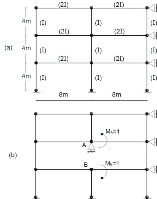
**Fig.5.** Numerical example (a) Braced frame, (b) Remainder frame.
