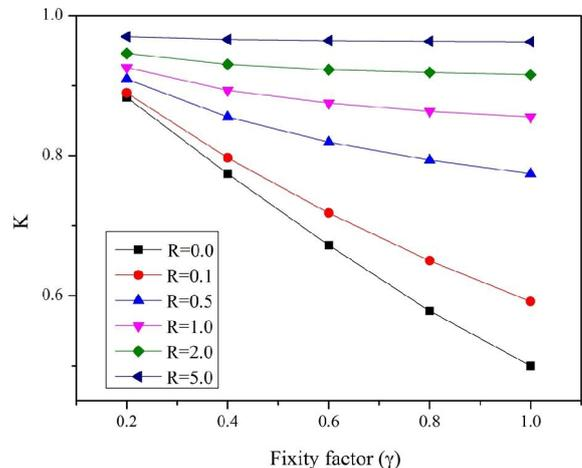
**Fig.4.** Braced effective length factor versus fixity factor ( $\gamma$ ).
