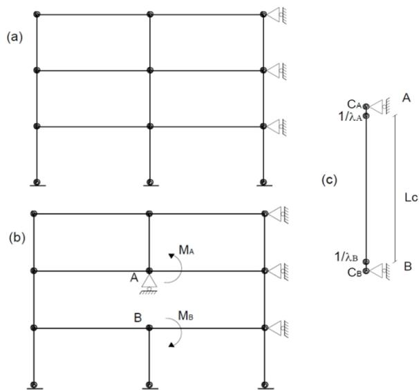
Fig.1. Braced frame (a), Remainder frame (b) and isolated member (c)
