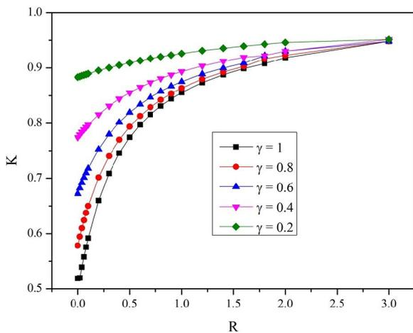
**Fig.3.** Braced effective length factor versus relative rigidity coefficient.
