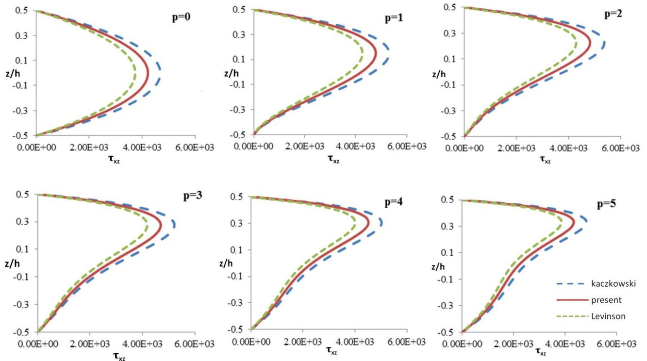
**Fig.11.** Variation of transverse shear stress across the depth of FGM beam under uniform load for different higher order shear deformation theory at  $(x=0)$  ( $L/h=5$ ).
