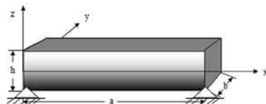
Fig.5. A functionally graded beam element in their axis
