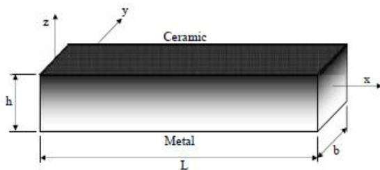
Fig. 1. An example of FGM beam Structure
