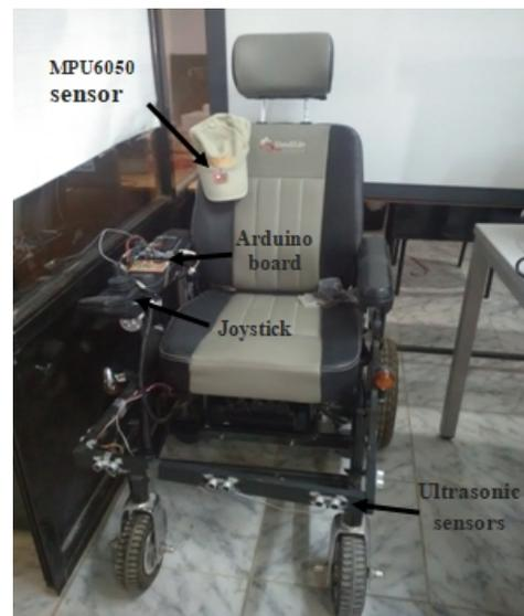
**Fig. 9 .** Hardware set up for the Intelligent Wheelchair
