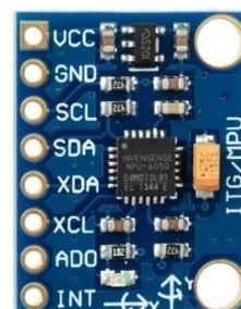
Fig. 2. MPU6050 IMU board.
