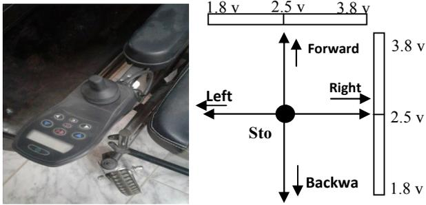
Fig. 3. The Joystick and the generated voltage from joystick axis.
